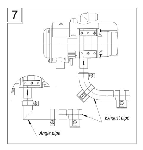
The exhaust pipe must be laid in a downward slanting direction from the pre-heater. If this not possible, then it is necessary to make a hole of size Ø3 at the lowest point for discharge of condensate.
